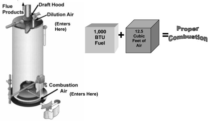
Do not forget that your gas (or oil) furnace and gas clothes dryer also require a like amount of air.
